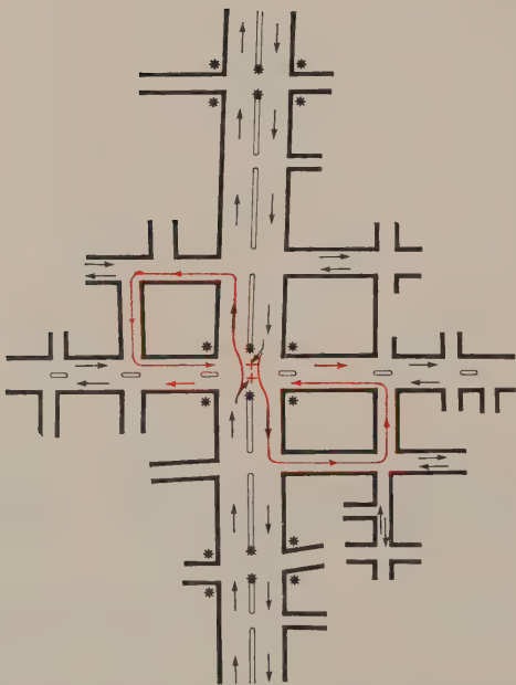
52 A typical traffic management measure. The difficult right-hand turns out of the main route are prohibited at the points marked by red crosses, and are replaced by left-hand turns which take traffic round the block (as shown in red) to a straight cross-over of the main route.
